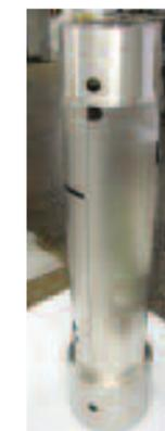
CRYOPERM™ 10 Magnetic shield Assembly for test cryostat (BESSY GmbH Berlin)
