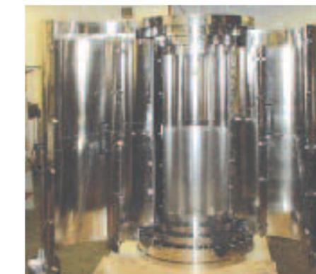
Four-layer AMUMETAL hinged-door Magnetic Shield Assembly for SQUID Microscope (California Institute of Technology)
