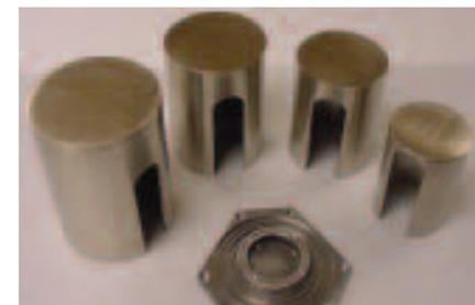
Multi-Layer Magnetic Shield Assembly to study nonlinearity associated with intrinsic magnetic characteristics of superconductors. Alternate layers of CRYOPERM™ 10 and AMUMETAL installed on ultra-low-carbon-steel base. (University of Maryland Physics Dept.)
